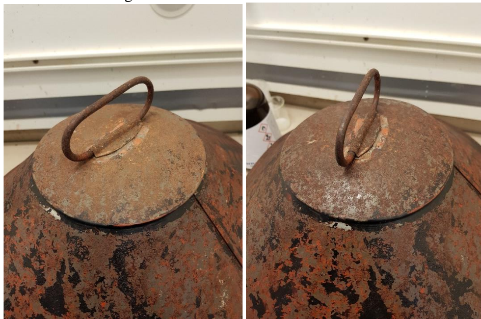
(Before an after of the Paraloid B44 lacquer)
